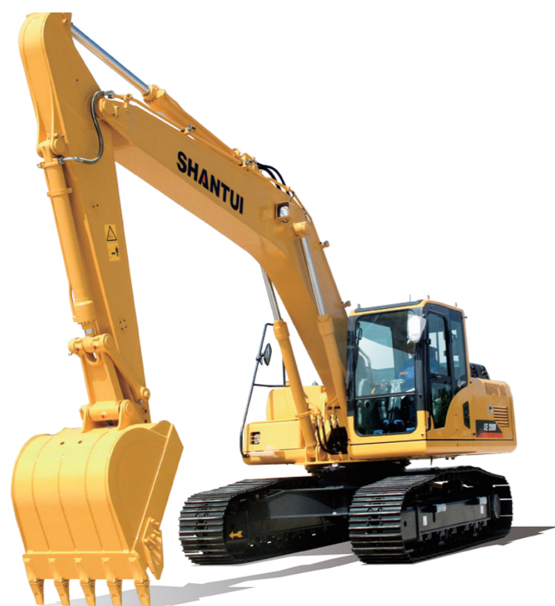
SE210 Tier 3 ▲ Rated Power: 116kW/2000rpm Engine Model: Weichai WP7 Operating Weight: 20500 kg
