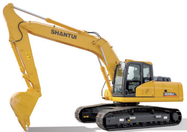
SE245LC Tier 3 ▲ Rated Power: 150kW/2050rpm Engine Model: Cummins QSB7 Operating Weight: 24800 kg
