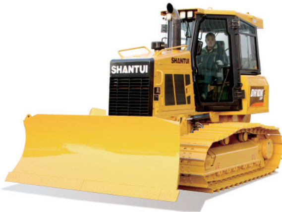
DH10K ▲ Use: General Net Power: 87kW/117HP/2200rpm Engine Model: Cummins QSB 4.5 Operating Weight: 10.2 Tons
