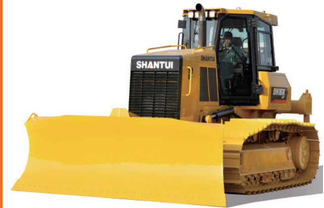
DH16K ▲ Use: General Net Power: 138kW/185HP/2000rpm Engine Model: FPT N67/ Cummins QSB 6.7 Operating Weight: 17.235 Tons
